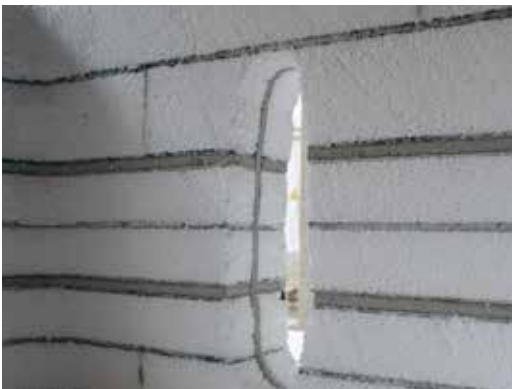
Styrofoam substructure with UHPC ribs
