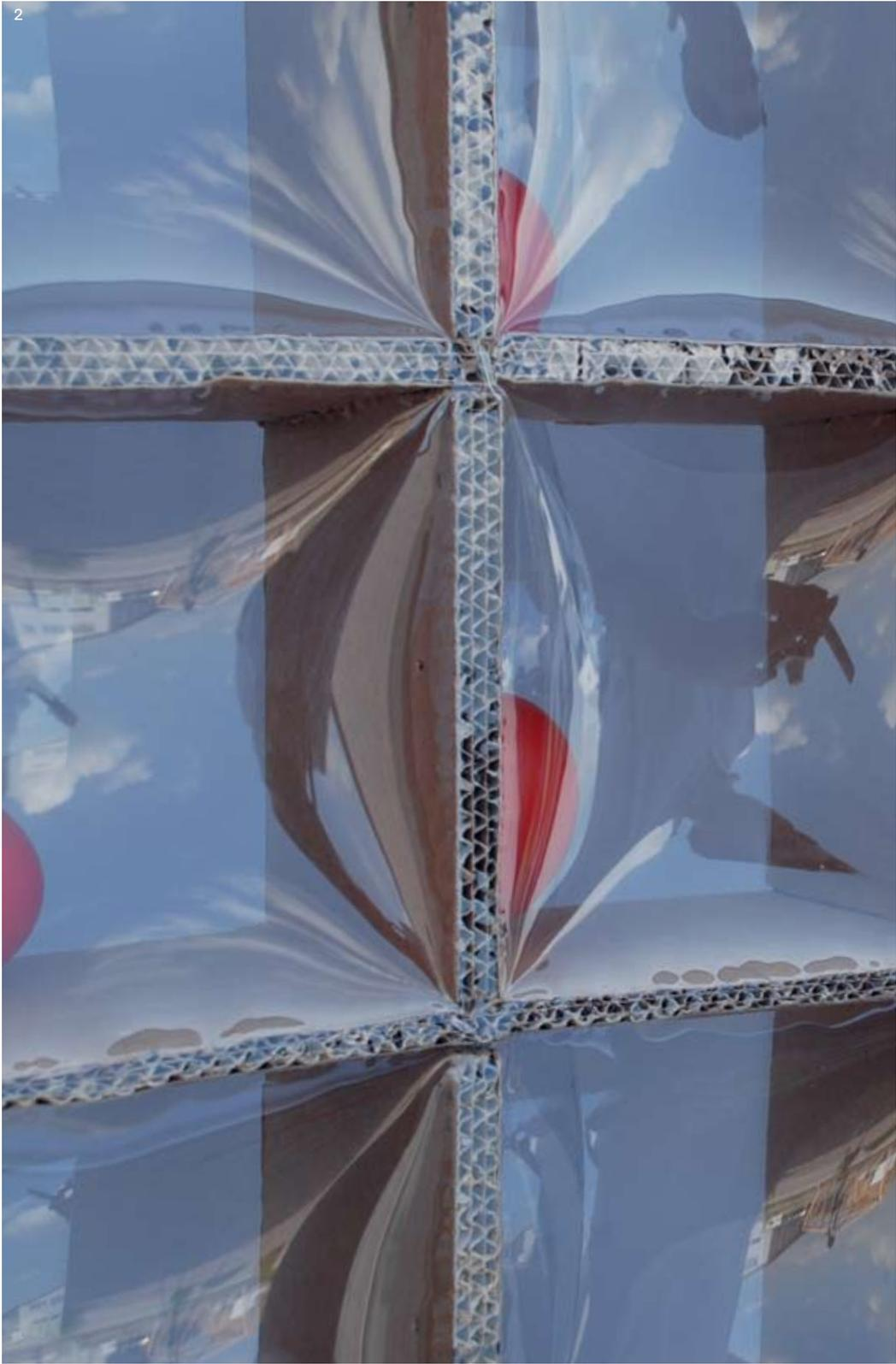
the cavity. For a cavity with a coarse vacuum of 0.1 bar, an improvement of up to approximately 10 dB(A) can be realized when compared to an ordinary situation under normal atmospheric pressure. Theoretically, even better sound insulation can be achieved with higher levels of vacuum.
