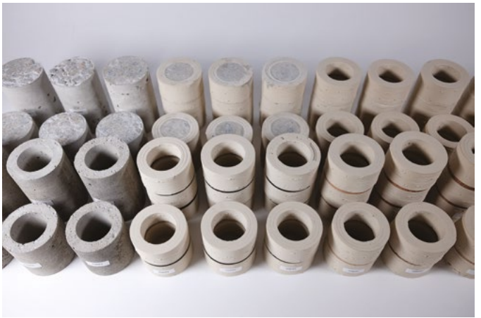
Figure 1: Complementary material specimens and concrete reference specimens for load bearing tests.
