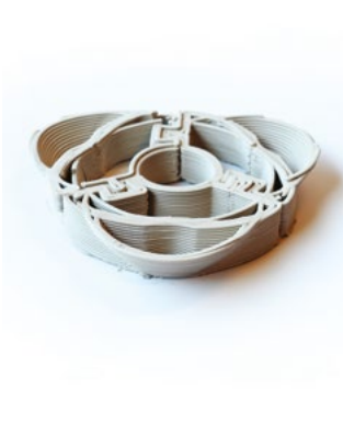
Figure 2: Three and four-part cladding prototypes, 3D clay printed (Photographer: Dena Khaksar).
