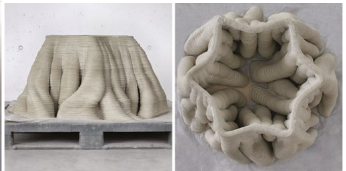
Figure 10: Artificial reef prototype printed in ceramic (left) and concrete (right).
