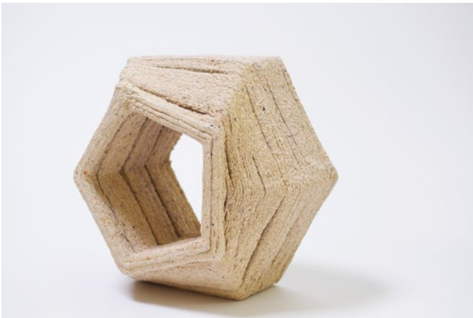
Figure 5: Shrinkage of Kusudama blocks. Delamination between layers due to evaporation of water.
