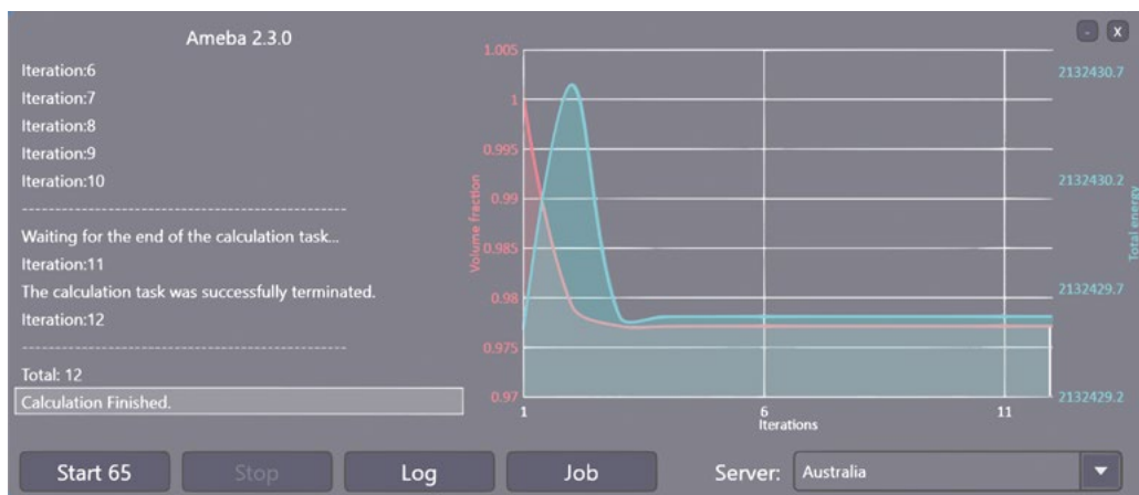
Figure 10: The initial spike in volume fraction quickly stabilizes, converging to approximately 0.975 by iteration 11, with total strain energy settling near 2.13 \times 10^4 .
