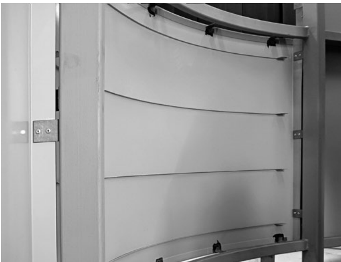
Figure 9: 1 mm steel plate reinforced with 4 ribs of 6 layers of 0.95 mm printed with WAAM. The reinforcement in turn generates the plastic deformation of the plate which follows a unidirectional curve with a radius of approximately 4 meters.
