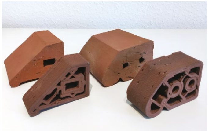
Figure 6: Profiled Bricks for cornices, lintels or pilasters.
