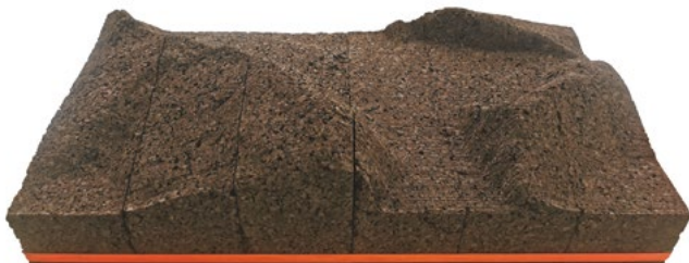
Figure 21: Artificial topography in cork produced through laboratory milling.
