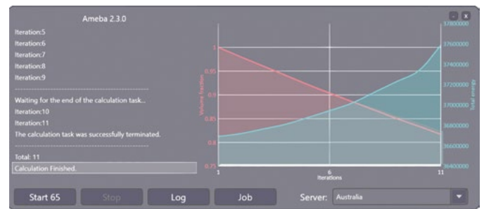
Figure 7: The final iteration achieves a volume fraction of approximately 0.95 while stabilizing the total strain energy near 3.74 \times 10^6 .
