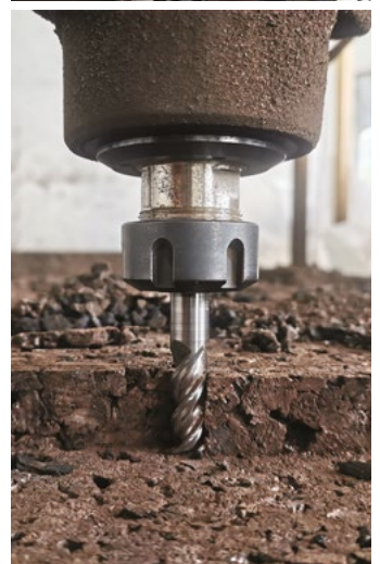
Figure 20: Milling process of the cork base.
