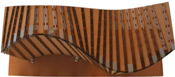
Figure 11: Laser cut prototype (scale 1:10) connected with hinges to reproduce a module of the outdoor installation.
