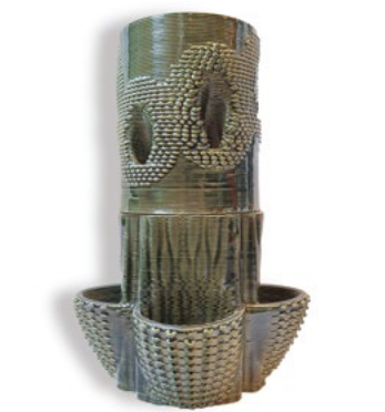
Figure 6: glazed and partially stacked 3D clay printed drum segments (Photographer: Dena Khaksar).
