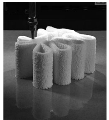
Figure 4: Pulpbaffle block after printing.
