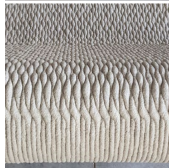
Figure 9: Concrete bench prototype - detail of the seam between layers (left) and full view (right).
