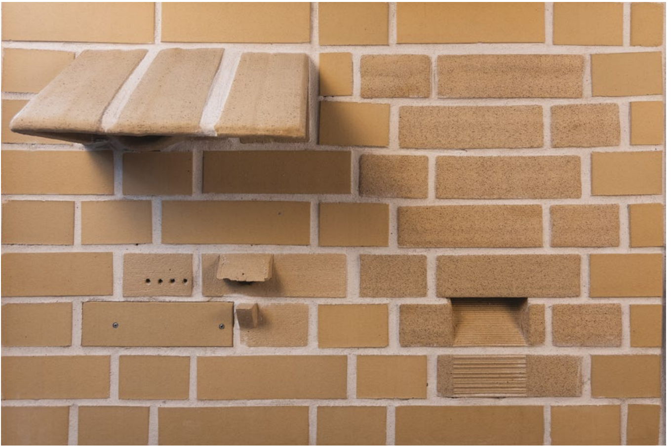
Figure 4: Three different Types of additively manufactured Nesting Bricks in a Demonstrator.
