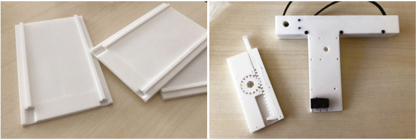
Figure 7: SLS 3D-printed solid PV modules and example of adjustment system components.
