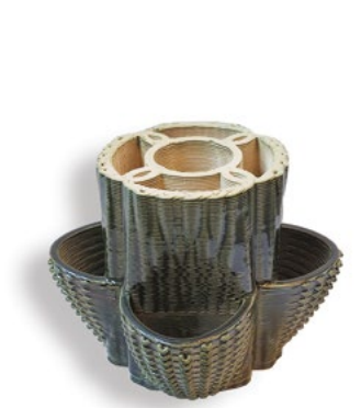
Figure 6: glazed and partially stacked 3D clay printed drum segments (Photographer: Dena Khaksar).
