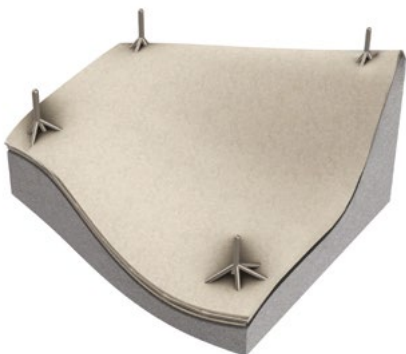
Figure 8: Final GRC Layer. Elaboration by the author.
