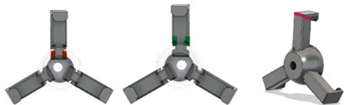
Figure 11: The potential failure points of the connection.
