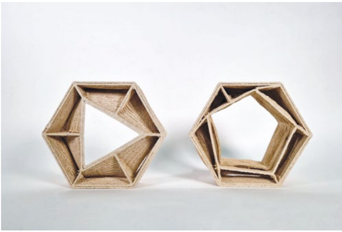
Figure 3: a) Study that determinates the maximum degree of curvature supported by the cellulose. b) Internal walls of the Kusudama Blocks.
