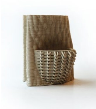
Figure 4: Singular cladding component showcasing ornamental computational patterns, 3D clay printed (Photographer: Dena Khaksar).
