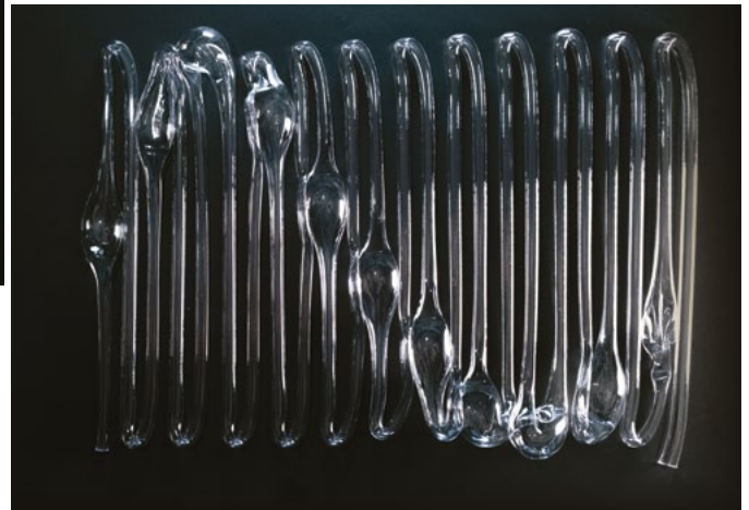
Figure 14: The results of blow extrusion in FGFBX procedure and PETG material varying the pipe diameter through variable material flow, air pressure. The hollow strands Diameter varies from 10mm to 45mm (Photo credit: Samim Mehdizadeh).
