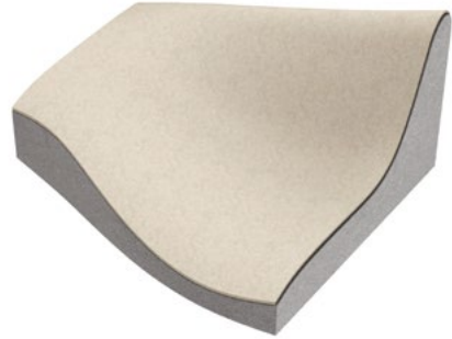
Figure 5: First GRC Spray Layer. Elaboration by the author.
