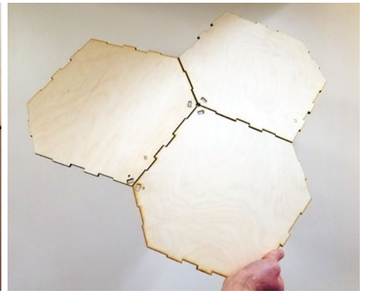
Figure 2: Friction fit connection system for the ECHO shell.
