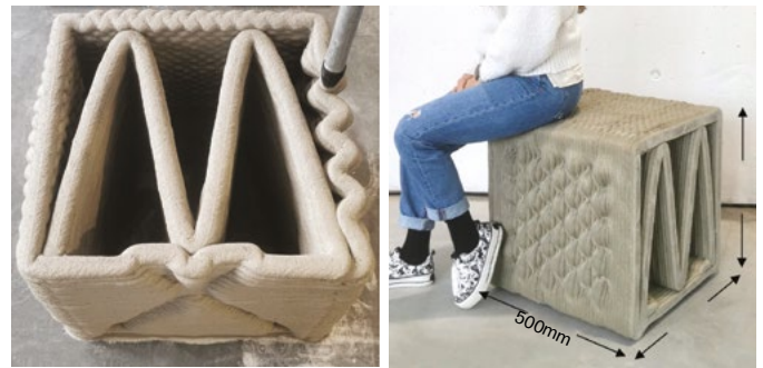
Figure 5: Demonstrator prototype with different textures and internal reinforcement.
