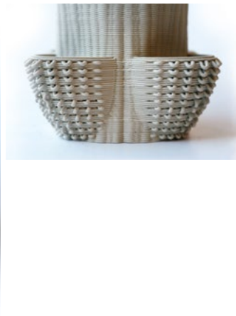
Figure 4: Singular cladding component showcasing ornamental computational patterns, 3D clay printed (Photographer: Dena Khaksar).
