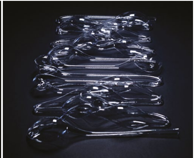
Figure 13: the results of blow extrusion in FGFBX procedure and PETG material varying the pipe diameter through variable material flow, air pressure. The hollow strands Diameter varies from 10mm to 45mm (Photo credit: Samim Mehdizadeh).
