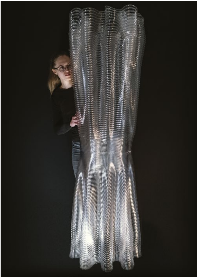
Figure 12: large scale Prototype Blow extrusion in two segments at maximum printing area of the robotic setup with UR10 robotic arm. Each segment of prototype is 1100 mm high and took about 300 minutes to print. Each segment only uses 5 Kg of PETG for print. (Photo Credit: Samim Mehdizadeh).
