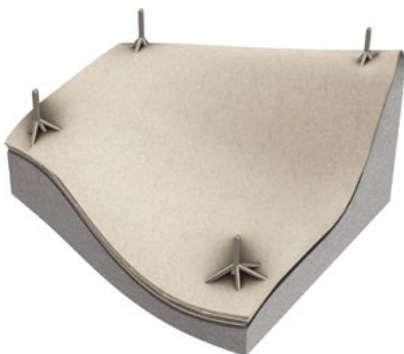
Figure 8: Final GRC Layer. Elaboration by the author.
