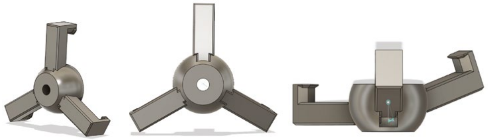
Figure 5: A standardized connection proposed for robotic assembly of shell systems.
