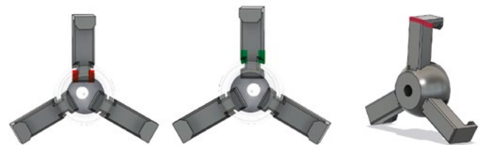
Figure 11: The potential failure points of the connection.
