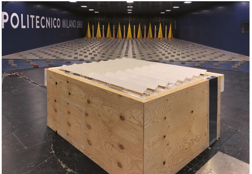
Figure 9: Scale model fully assembled inside PoliMi boundary layer wind tunnel.
