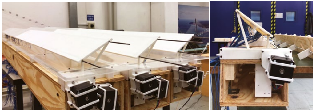
Figure 8: Scale model strings assembled and equipped with stepper motors for adjustment capability.
