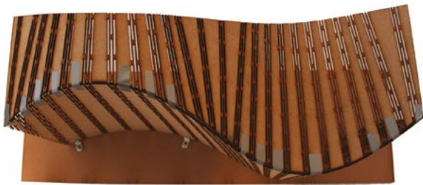
Figure 11: Laser cut prototype (scale 1:10) connected with hinges to reproduce a module of the outdoor installation.
