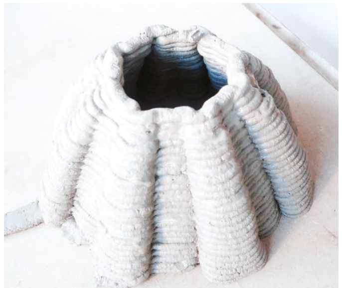
Figure 12: Extrusion test of a 1:10 scale shell geometry using a 15 mm nozzle, based on a rib-reinforced computational design method.
