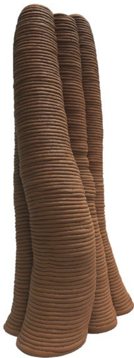
Figure 11: Scaled prototype 1:10 3D printed using a laboratory robot at IAAC Institute for Advanced Architecture of Catalonia and nozzle 25mm, demonstrating controlled cavity design to reduce buckling and displacement.
