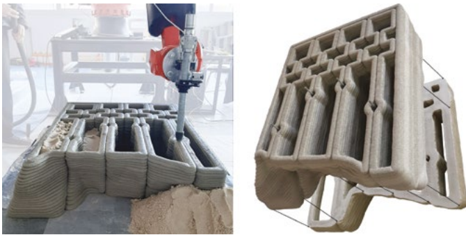
Figure 19: Printing process of a full-scale prototype (a) and post-tensioned assembly of two printed sections (b).
