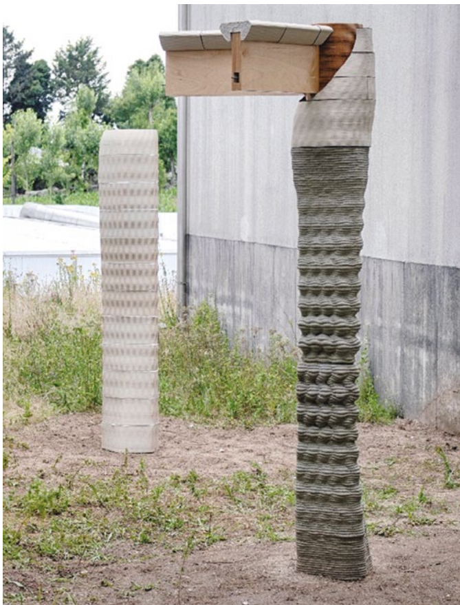
Figure 6: Comparison between the ceramic column composed of twelve segments and the concrete column composed of two segments.
