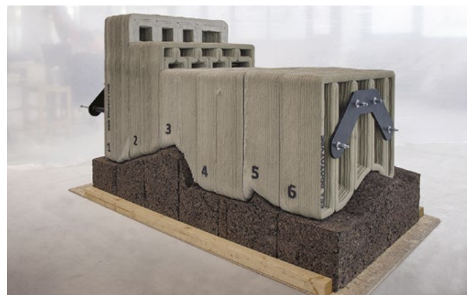
Figure 22: Fully assembled prototype in the ARENA Laboratory after post-tensioning application.
