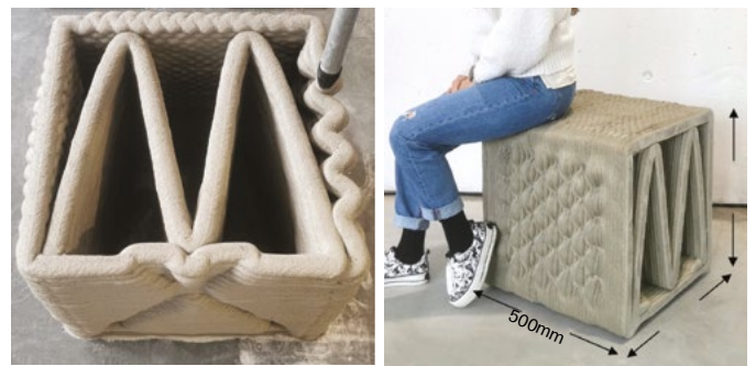
Figure 5: Demonstrator prototype with different textures and internal reinforcement.
