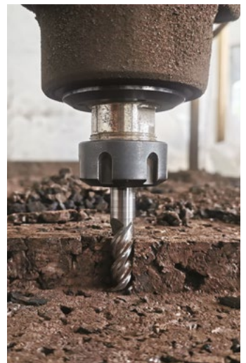
Figure 20: Milling process of the cork base.
