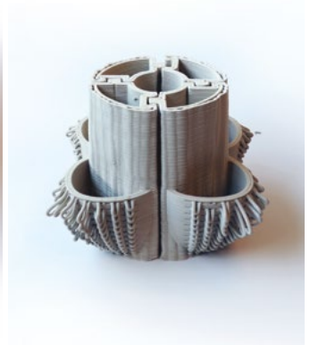
Figure 3: Four-part cladding prototypes, 3D clay printed, (Photographer: Dena Khaksar).
