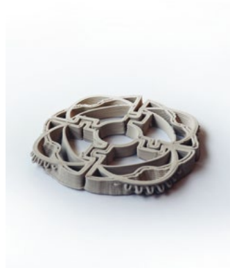
Figure 2: Three and four-part cladding prototypes, 3D clay printed (Photographer: Dena Khaksar).
