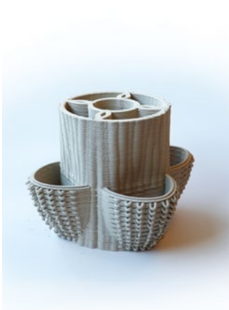
Figure 5: circular 3D clay printed drum segment (Photographer: Dena Khaksar).
