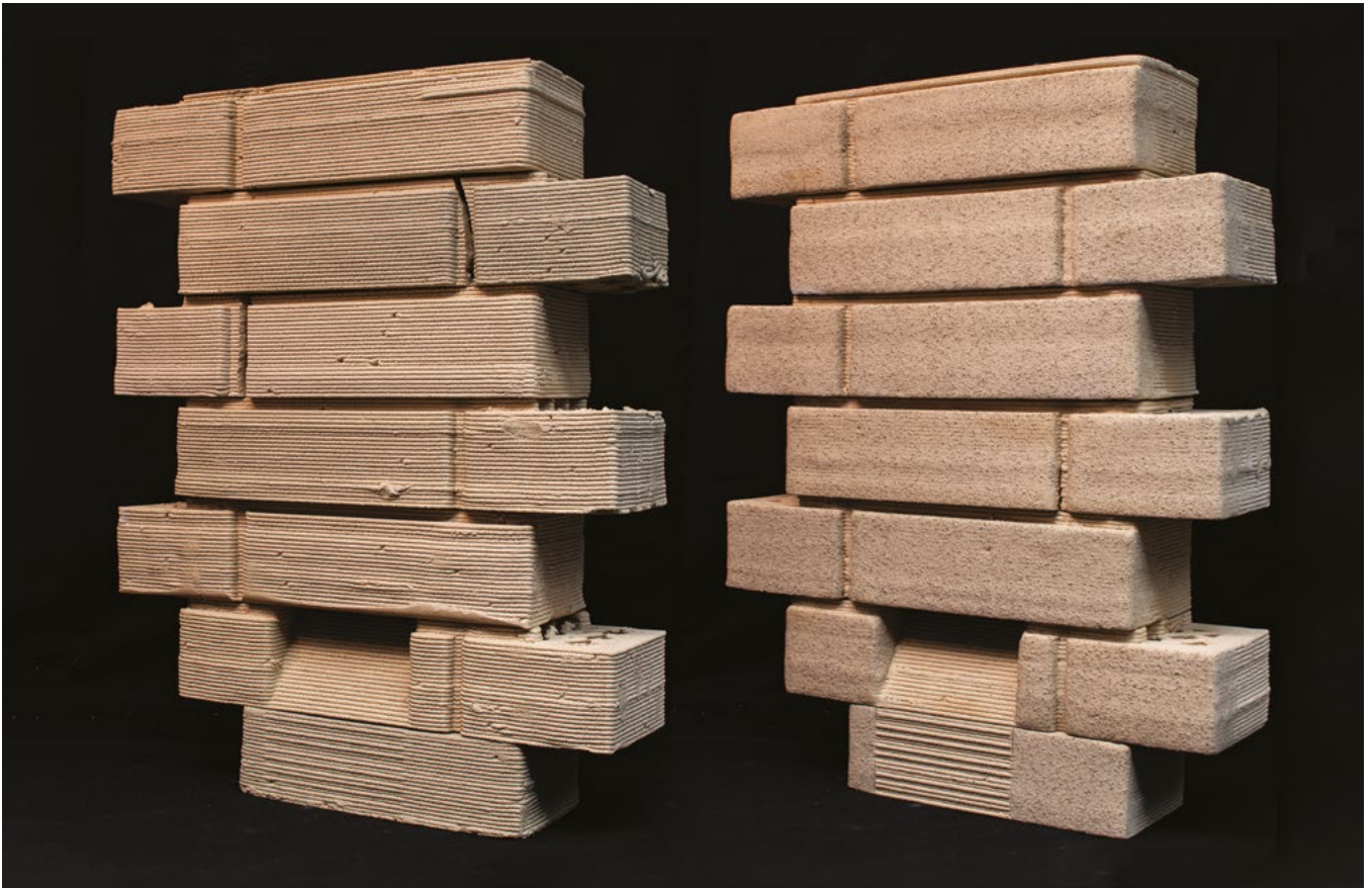
Figure 5: Directly printed and optimized Nesting Brick in comparison.
