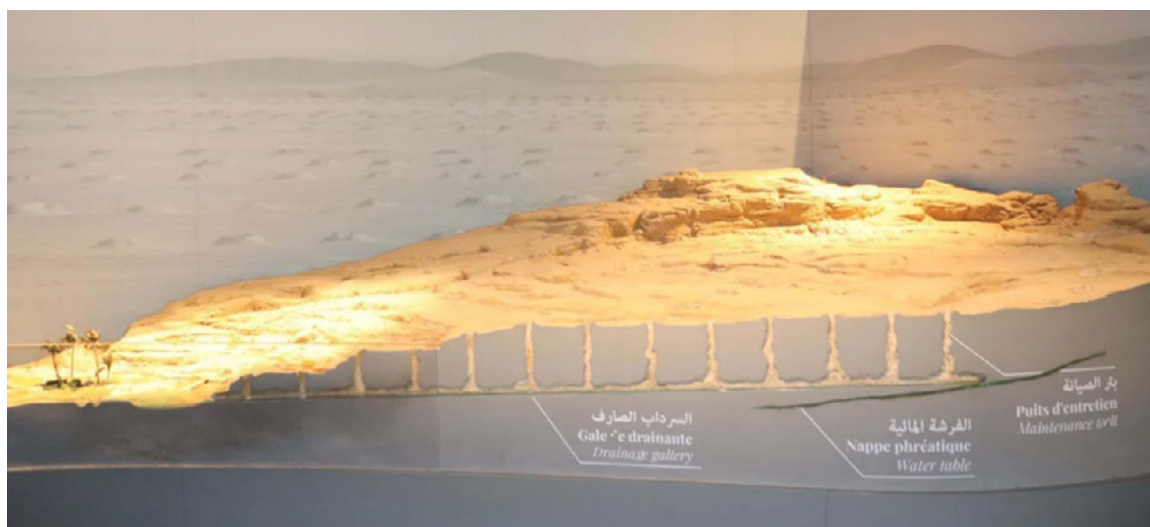
^ Fig. 2 A diorama inside the Aman Museum showcasing and labeling in three languages the underground components of a khetarra : a long gallery that taps into the water table and angles down toward an irrigation field or oasis community, and several maintenance wells that can be accessed from above ground. (Source: Cristiana Strava, 2023).
