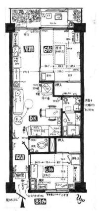
Figure 22 Drawing of the floor plan of a post-war high-rise apartment (47m²) that belonged to Nishiyama's friend K in 1967, featuring two tatami rooms and the use of each space, published in his series on housing in Japan (Source: Uzō Nishiyama Memorial Library)
