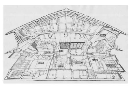
Figure 6 Nishiyama's innovative depiction of a traditional Japanese house from above, depicting both the architectural structure as well as the use of the various spaces. Transforming lifestyles are captured through the presence of a piano in the room at the lower left (Source: Uzō Nishiyama Memorial Library)
