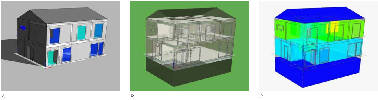
FIG. 5.1 Presentation of the building's model (A), its energy interpretation (B), and graphic presentation of the result (C)
