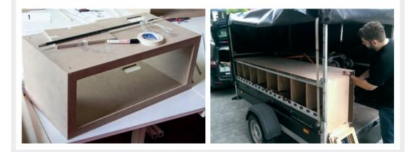
of the frames were subject to various requirements: they had to be combinable so that several results could be merged into one prototype in efnMOBILE format. In addition, transportability and affordable production were important prerequisites. Therefore, MDF boxes (dimensions: height 30cm, width 74cm, depth 38cm) were built at the University of Applied Sciences Detmold as templates.
