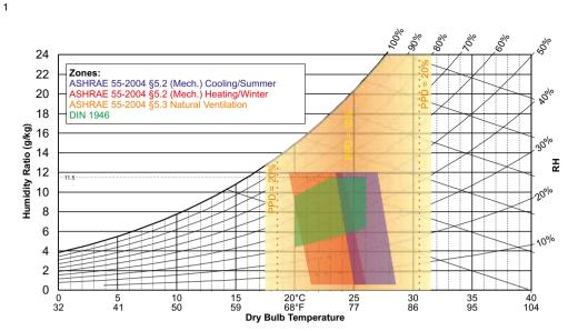
NOTE: Natural Ventilation zone depends on mean monthly outdoor temperature. Zone, as shown, only represents potentially acceptable temperature ranges for comparison to the traditional standards of mechanically-ventilated zones. Darker area in this zone shows temperatures with wider range of outdoor temperatures (yellower extremes only acceptable near 10°C or 33°C outdoors). Read §5.3 before applying!
